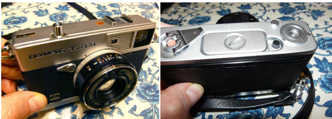
Figure 12 – Left: Example of the Olympus 35 ECR camera Meier used for these photographs; Right: Camera underside showing film release button, tripod mount and rewind lever on the base.
